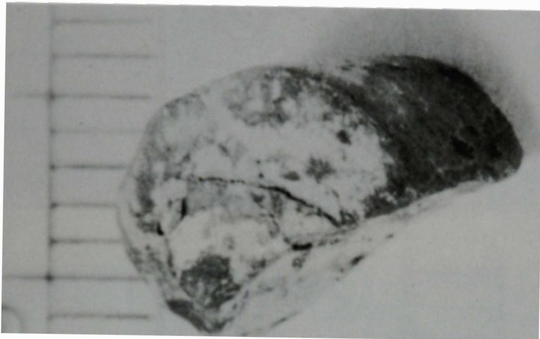
Figure A-14. Particle 4U from Sample 4 (surface of debris bed at E9 location), size range:  $>4000 \mu\text{m}$ .
